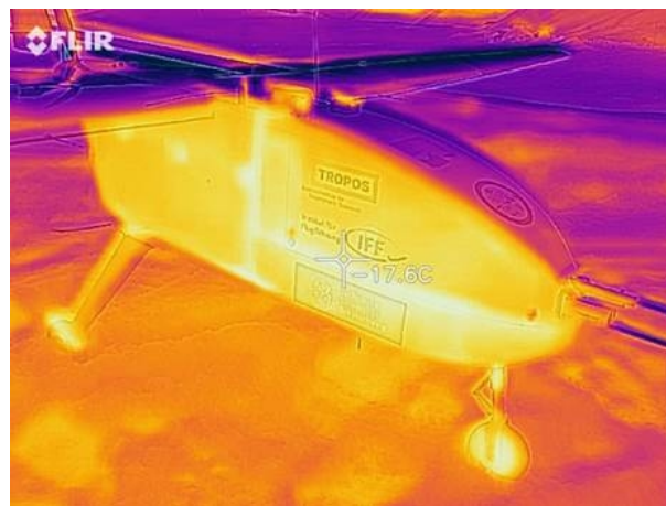
Figure 4. Thermal infrared image of ALADINA. The thermal bridges are visible at the intersections of different compartments and were responsible for losses of heat during the flight.
