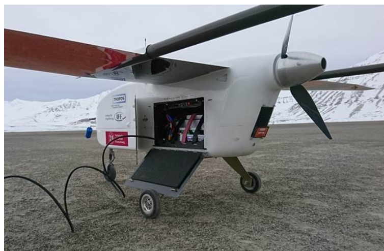
Figure 3. ALADINA during turnaround and saving data via downlink. The battery is stored in the back of the payload bay and can be removed easily by opening the side door. The full compartment was insulated. Photo: Alexander Peuker, TU Braunschweig.
